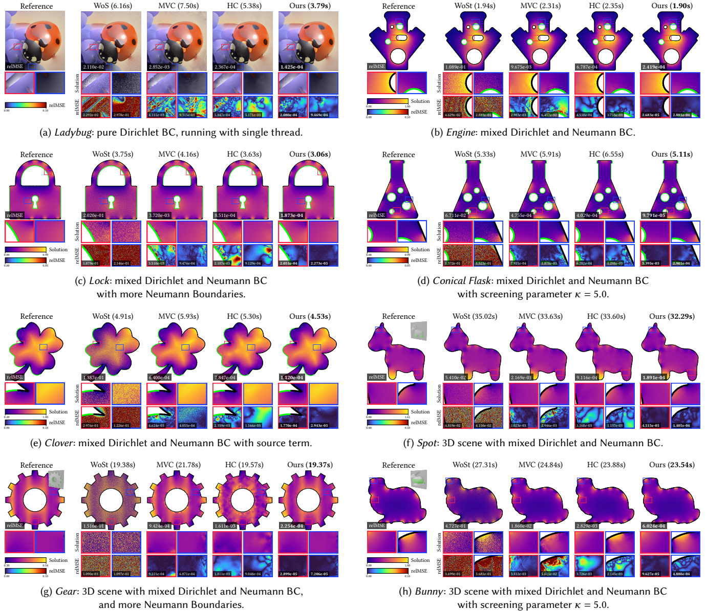
Fig. 11. Comparison of variance reduction techniques across various 2D and 3D boundary value problems. For 3D scenes, we set query points only on the interested planar. For MVC, we follow the adaption described in [Zhou et al. 2025, Appendix E] to handle screened Laplace equations.
